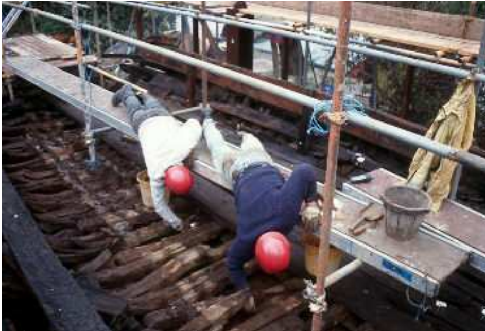
WS29 The careful inspection and initial preservation work of “Dee Dar’s” remaining timbers.
